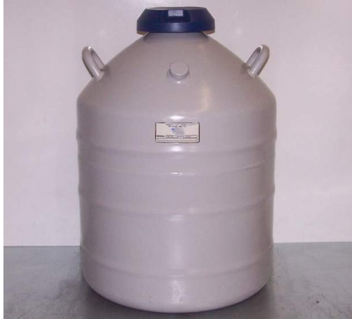
Fig. 4. Liquid nitrogen Dewar vessel, used for freezing and storing cryopreserved oocytes. Courtesy of Reproductive Medicine Associates of New York, LLP.
